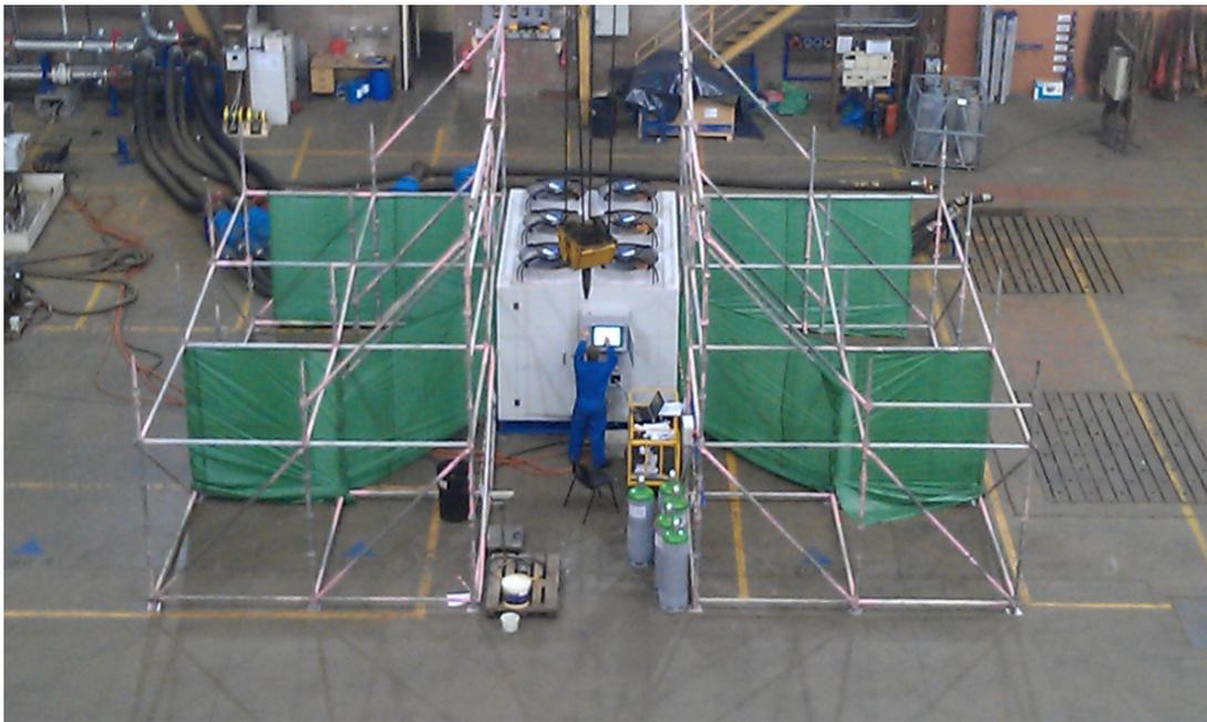
**Figure 5 – chiller test set up (without the top tarpaulin).**
