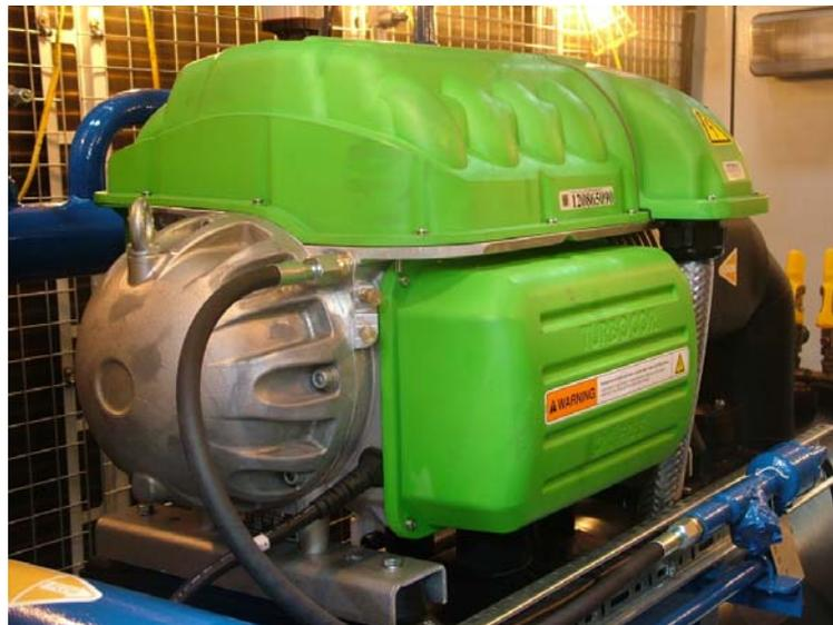
**Figure 3 – Prototype compressor for HFC-1234ze(E).**
