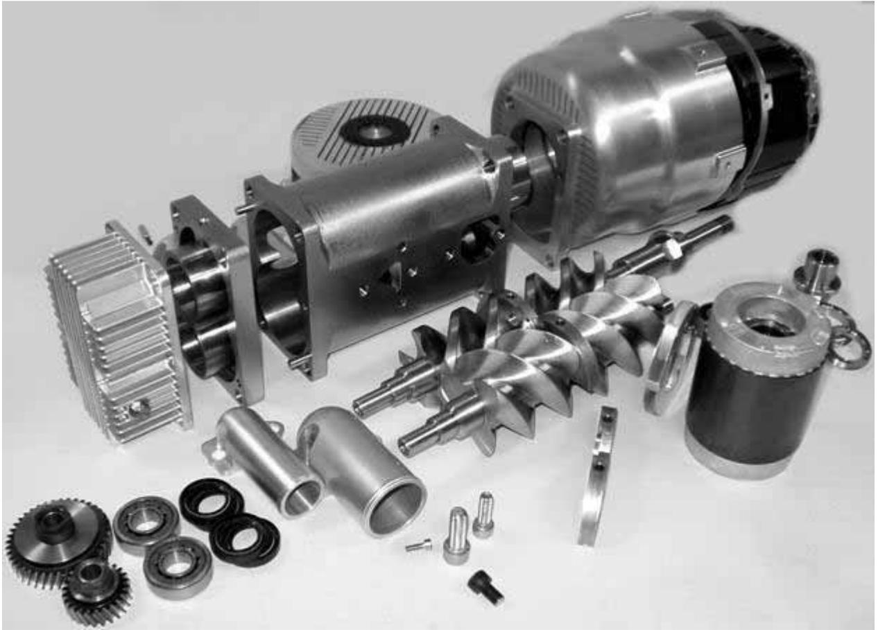
**Figure 17 Screw machine for simultaneous compression and expansion**
