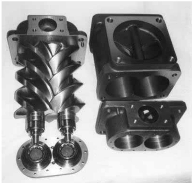
**Figure 18 The 'Expressor' principle and the first prototype machine**
