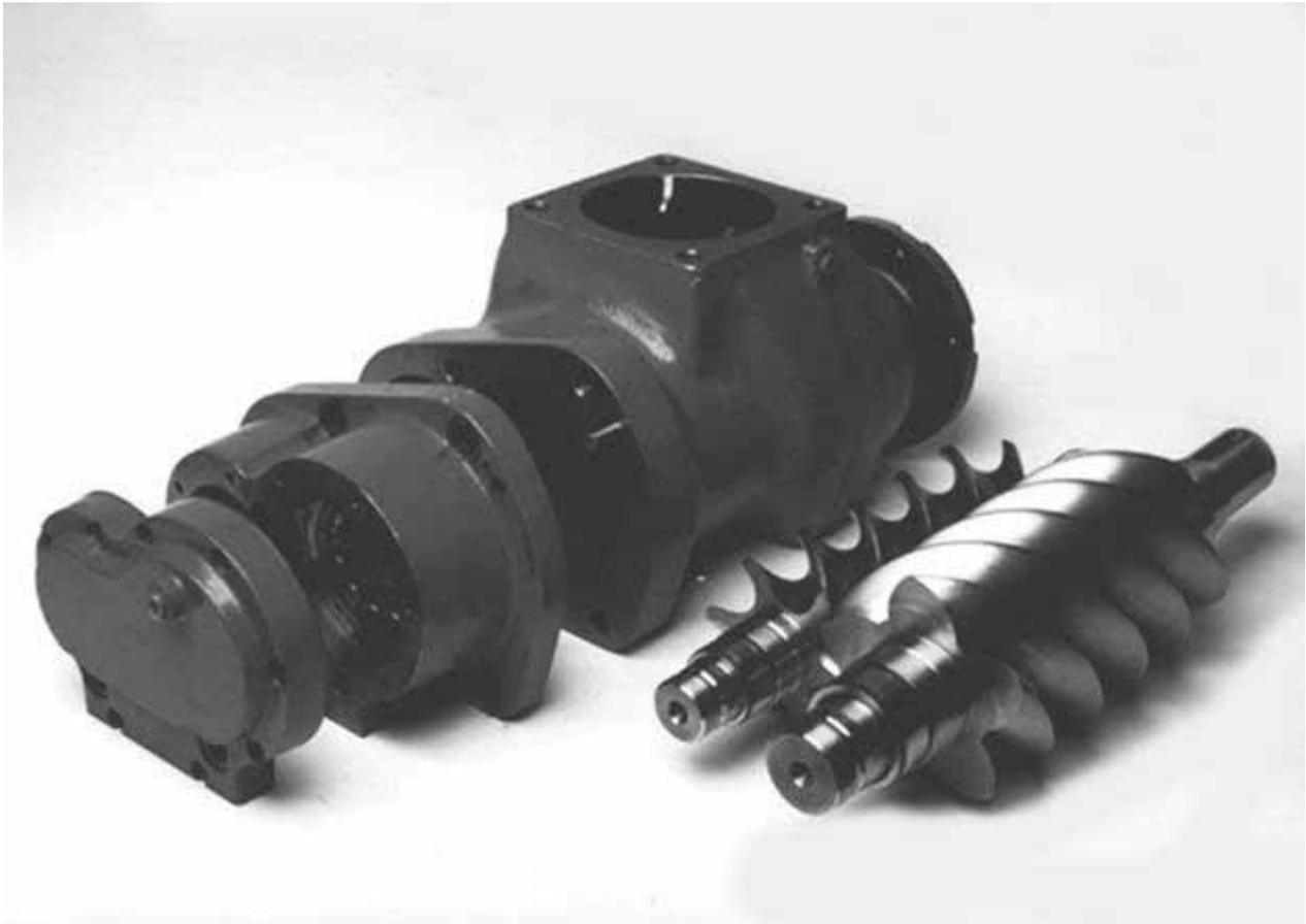
**Figure 2 Screw compressor main components, rotors and housings with bearings**
