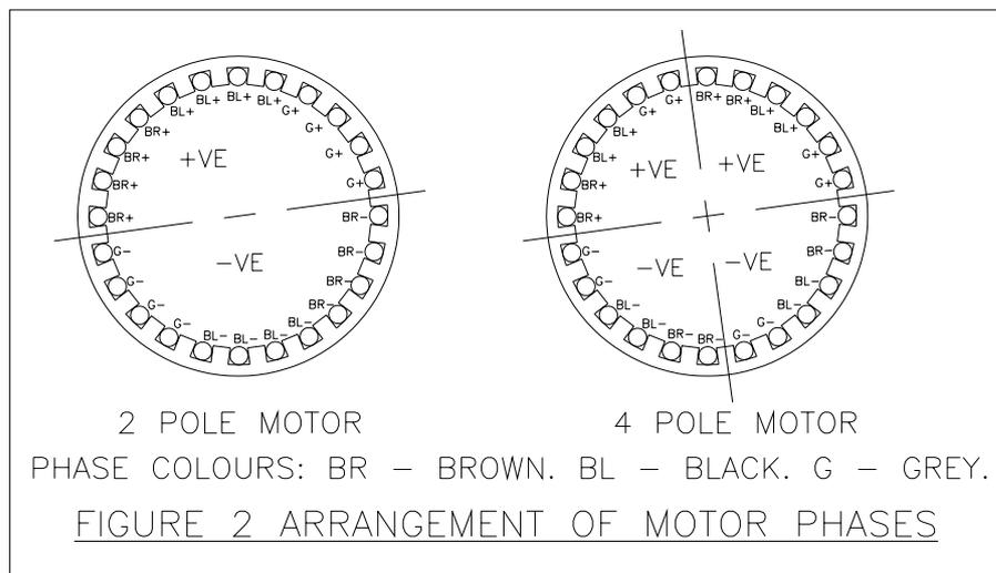
The way in which the windings are connected will determine the speed at which the shaft rotates. The simplest (and fastest) induction motor has only one pair of magnetic poles per phase and rotates once for every cycle of mains voltage. Hence, on a 50Hz supply it will run at just below 3000 rpm. Note that if the windings are connected to give a greater number of pole pairs, the motor will run more slowly but there are just as many windings (Fig 2).
